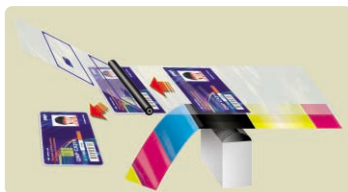
Re-Transfer printing process
